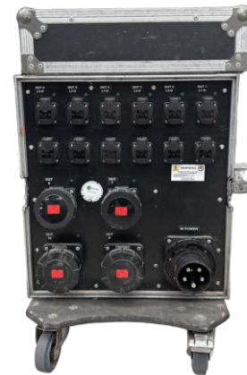
Rack 125A – 2x63A – 2x32A – 6x16A
